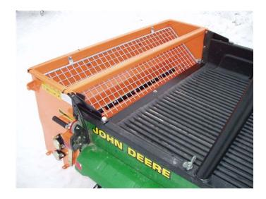
Designed for the JD Gator. Electric drive(also available w/hydraulic drive). Mounts on rear of box in place of tailgate. Dump box feeds material into hopper. - Hopper capacity - 180 ltr - Spreading distance w/salt - 4 km -Spreading distance w/salt - 4 km -Spreading distance w/salt - 0.8 km -Weight - 80 kg (176 lbs) - Spreading width - 1260mm (49") - - Screen -Roller with 5/3mm changeable cams -Agitator - Handle for output adjustment.
